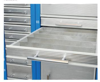
Each drawer is electromechanically locked and is unlocked by the software after entering the item to be taken out. A drawer can be used as a large single compartment for long tools, e.g. measuring tools, assembly tools, drilling tools, etc.
